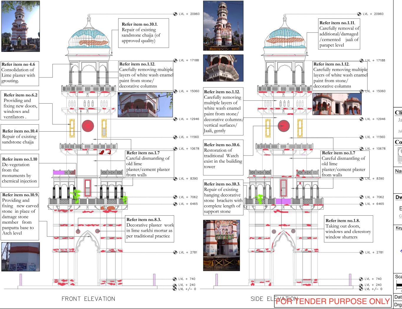
LEGEND Structural cracks Minor /Hairline cracks Soot deposit Missing plaster exposing masonary Buldging of Plaster Flaking of stone/plaster Water seepage Dampness Microbiologica arowth Damaged masonry/floor Damaged members Blocked opening Vegetation Missing elements Addition, alteration on walls & floor Multiple layer of enamel paint Cement plaster Debries/Malba/ Deposit Earthfill
